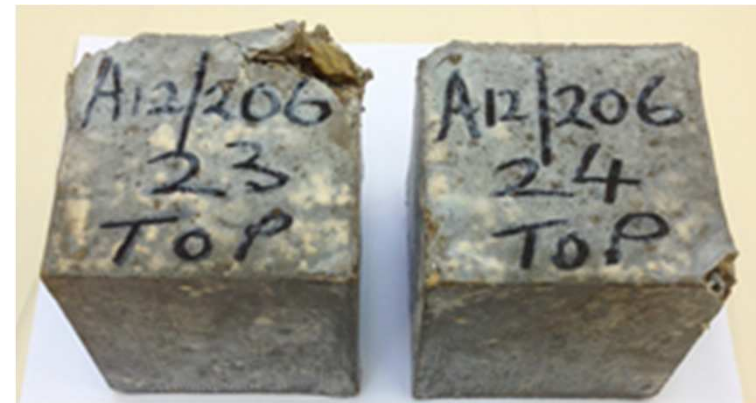
PC concrete 300 kg/m 3 and free w/c 0.50 after 2 years
